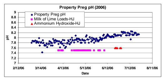
Figure 10: pH changes in the pregnant solution with to milk-of-lime and ammonium hydroxide injections into the heap interior via Hydro-Jex (Seal, 2008)
