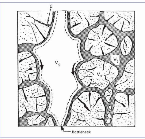
Figure 1: Schematic image of rock particles (V<sub>s</sub>), microporosity (ε), solution film (V<sub>l</sub>), void (V<sub>g</sub>) space, (Bartlett, 1998).
